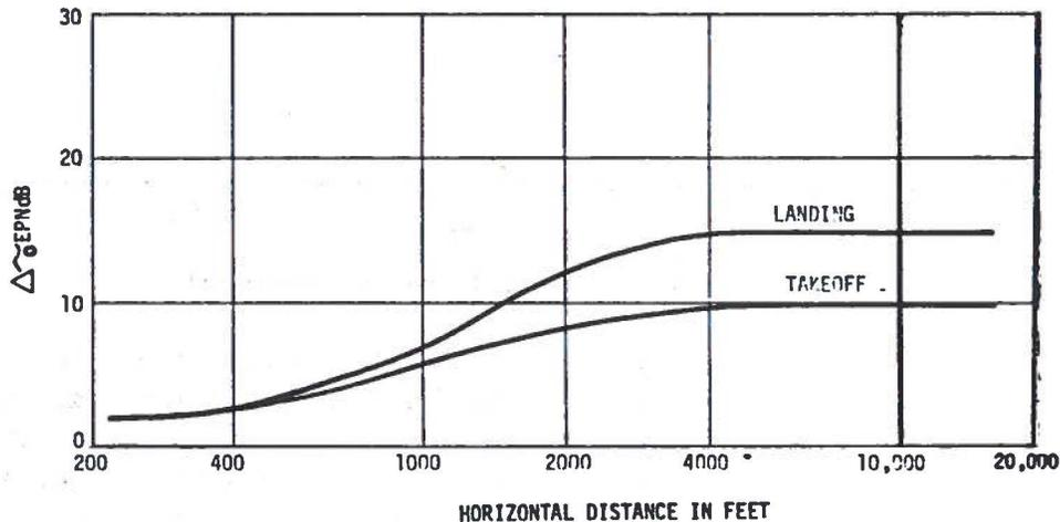
FIGURE 1 - Approximate addition attenuation for ground-to-ground aircraft noise propagation
