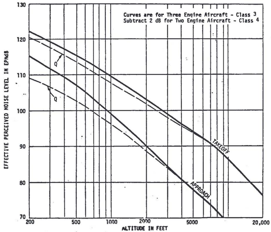
FIGURE E-3. Variation in effective perceived noise levels with altitude
