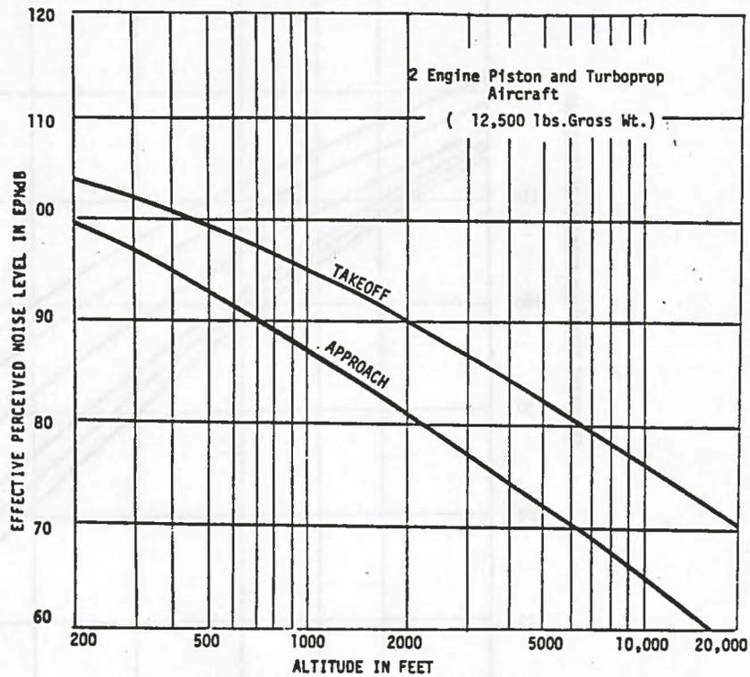
FIGURE E-5. - Variation in effective perceived noise levels with altitude
