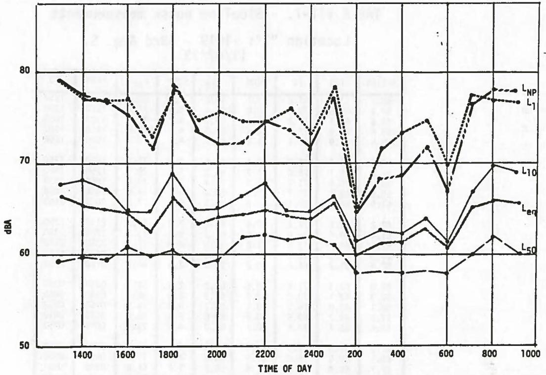
FIGURE N - Statistical levels measured at one sideline position
