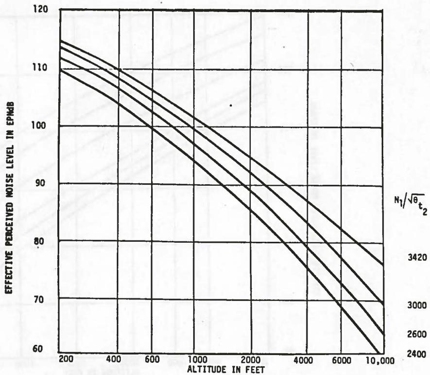
FIGURE F-5. Noise-Thrust-Altitude curves for Class 6 aircraft
