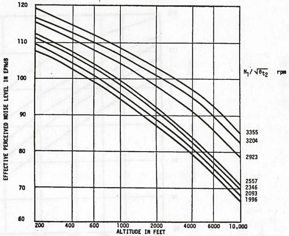
FIGURE F-4. Noise-Thrust-Altitude curves for Class 5 aircraft
