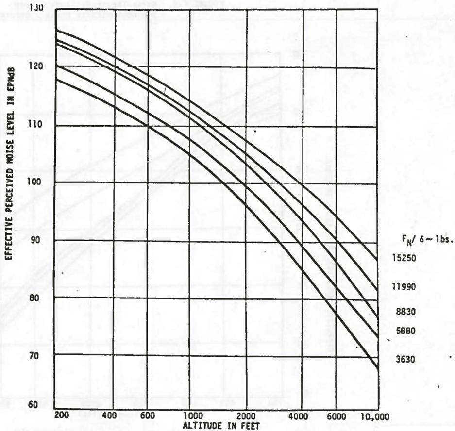
FIGURE F-1. - Noise-Thrust-Altitude curves
