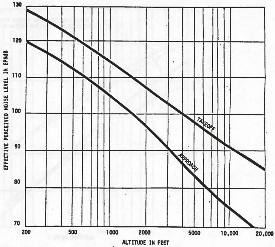
FIGURE E-1. - Variation in effective perceived noise levels with altitude
