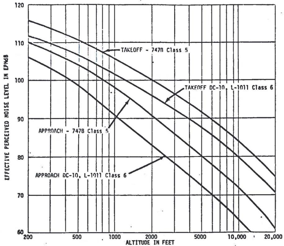
FIGURE E-4. - Variation in effective perceived noise levels with altitude
