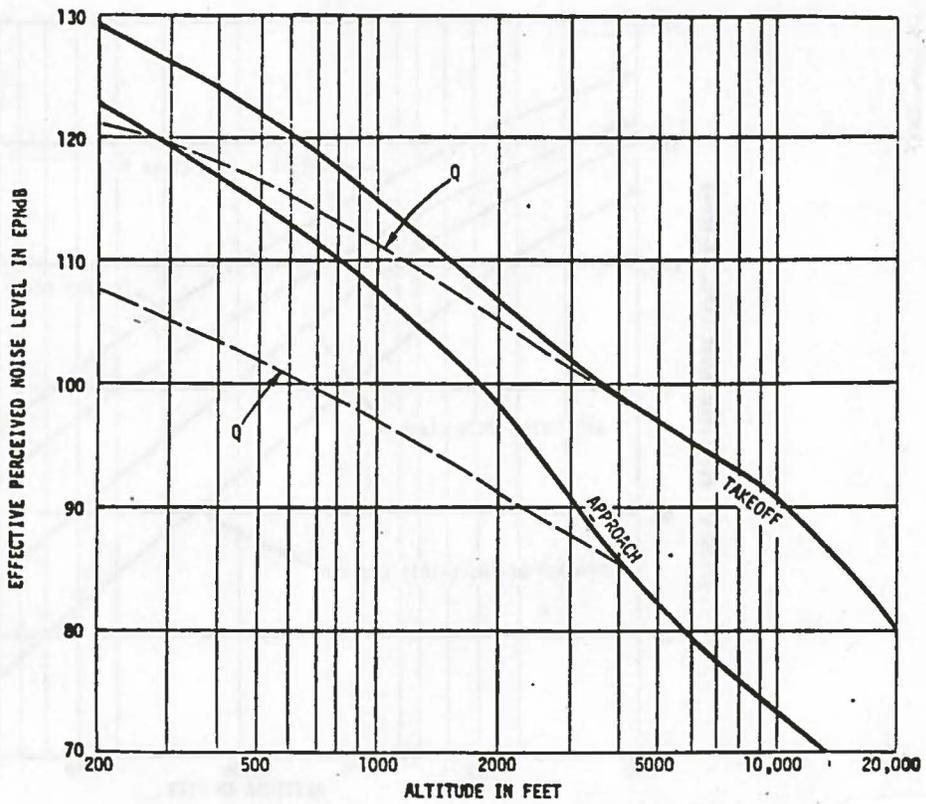
FIGURE E-2. - Variation in effective perceived noise levels with altitude
